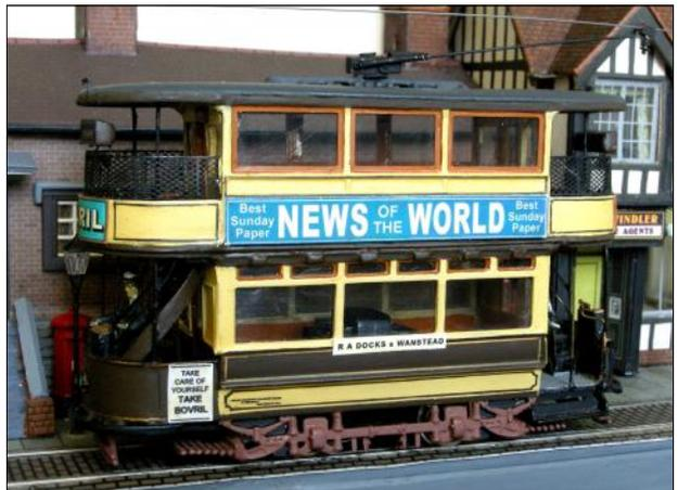
**Ex-Ilford 40** was built as a static model from a modified ABS white metal kit and was unsuitable for my East London Layout having no conduit. It represents the car in 1938. For this project I have motorized it with a Tenshodo motor unit and fitted a Meadowcroft working trolley pole.
