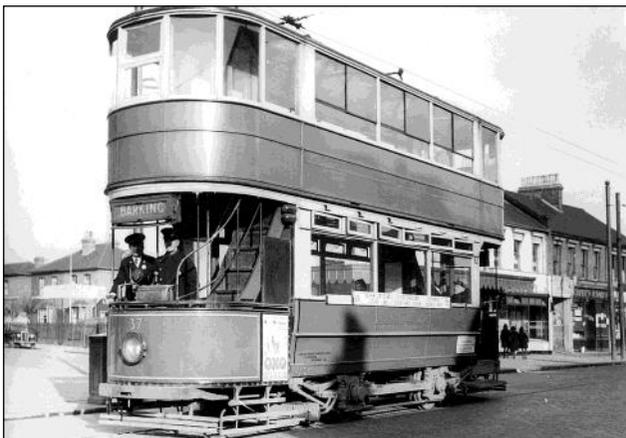
When the LCC was operating the **Leyton system** they had transferred in a number of M class cars to replace the life expired Leyton 4-wheelers on the local routes. The practice continued in LT days and car 1677 moved to the West Ham depot in 1935 and is seen here at Stratford Broadway. The original car was built by Hurst Nelson in 1910 on a Class 5 swing-bolster truck. London Transport retained the fleet number and it ran until 1937.
