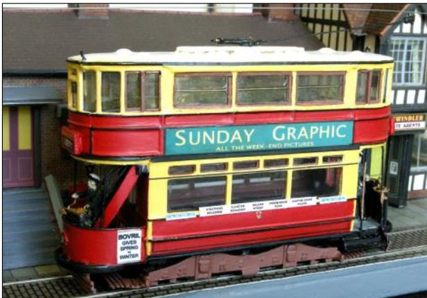
**London Transport 2039 ex-Walthamstow** is a completely new model built recently from an old BEC kit with a bit of modification. It is modelled in its final form at the end of 1936. It is fitted with two Meadowcroft trolley poles.
