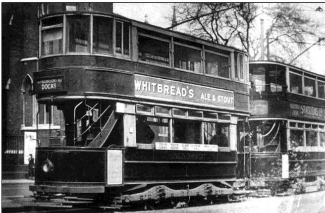
This is one of a group of 32 open-top cars built in 1905 by Brush and on Brush 21E style trucks as **Walthamstow 21**. It received the top cover and double trolleys in 1928 and was rebuilt in the "six-window" form in 1931. It is seen here as LT 2034 in Markhouse Road. It ran until January 1937.
