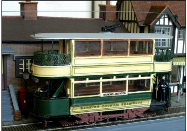
**Ex-East Ham 37G** was modified from a BEC white metal kit many years ago and modelled in 1934 condition for occasional use on my East London Layout as a "Special". It was conduit fitted, but for this project I replaced the dummy trolley pole with a Meadowcroft working one.
